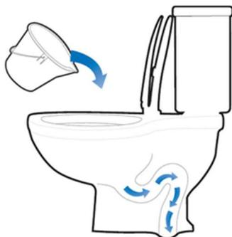
Flush toilets have a tank and pour flush have no tanks. But flush toilet with a tank can act a pour flush but not the other way around.
