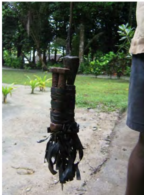
Figure 2.9: Hand-made torpedo line to pick-up bêche-de-mer at greater depth (15–18 m).
